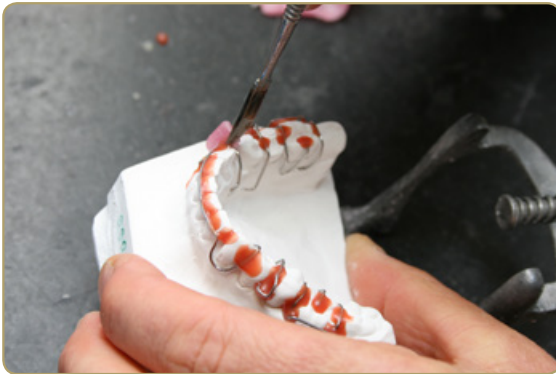
Fig. 5: Clasps and labial arch are fixed on the model with hot wax.
