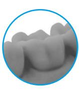
Surface with ± 50 µm Z-resolution
